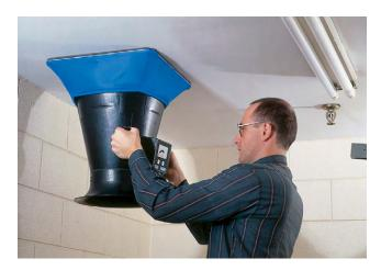
The LoFlo Balometer® Capture Hood is mainly used in residential or light commercial applications for taking measurements from 10 to 500 cfm (17 to 850 m<sup>3</sup>/h). The compact size allows them to be used where full size hoods would not fit such as over bathroom stalls or filing cabinets.
